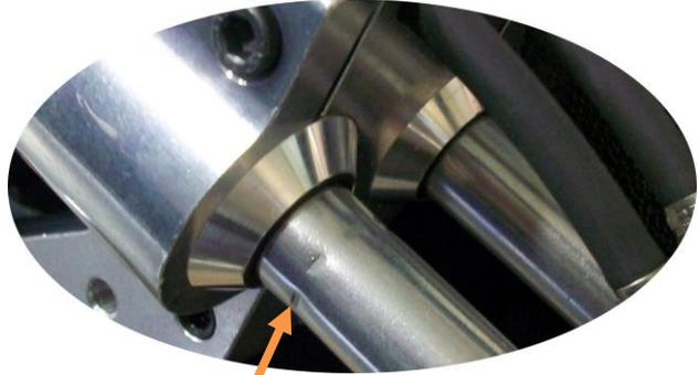
THIS LINE SHOULD COMPLETELY DISAPPEAR WITHIN THE GUN HOUSING WHEN THE GOOSENECK IS FULLY INSERTED.
