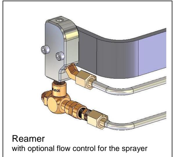
**NOTE:** Choosing Reamer option 'C' - Flow Control adds an adjustable check valve, giving users the ability to control the amount of TOUGH GARD Anti-Spatter applied in each spray.
