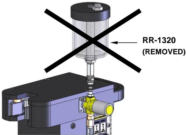
All Reamers are multi-feed ready by removing the sprayer reservoir (RR-1320) since it is not needed with the Multi-Feed System.
