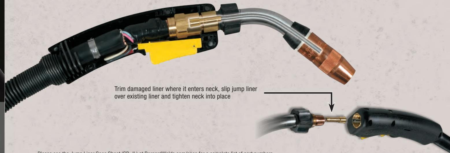
Trim damaged liner where it enters neck, slip jump liner over existing liner and tighten neck into place
