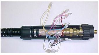
Insert spring into spring groove at the rear of the handle and tuck connected switch leads into handle.
