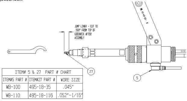
Step #6 Reinstall and tighten retaining head and contact tip and slide on nozzle.
