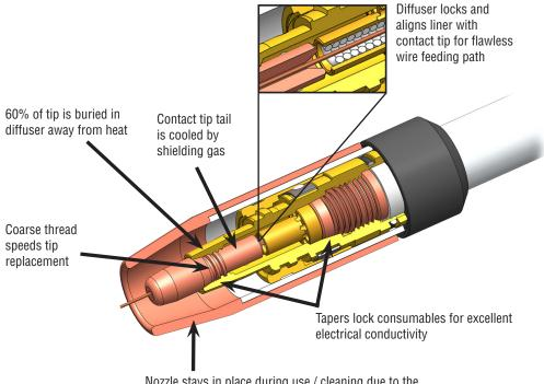
Nozzle stays in place during use / cleaning due to the steel retaining ring on the diffuser that helps to keep the threaded nozzle from loosening
